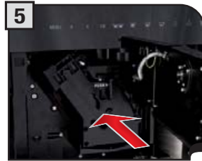
5 Fit it back in the machine. Do not press the "PUSH" button.
