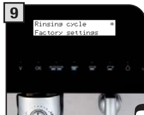
9 Press the "MENU" button. Select "Rinsing cycle" using the "v" or "Λ" button.
