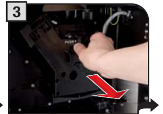
3 Press the PUSH button to remove the brew group.
